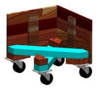
After cutting the two pieces of the x-brace (A) to 20 inches cut the corners of each board off at a 45 degree angle. Once all the corners are removed the boards should look like an arrow with a point on each end of the board.
