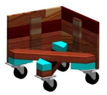
**3.** The four small boards (B) should have one end cut off at a 45 degree angle. The longest side of each board should measure 7 inches.
