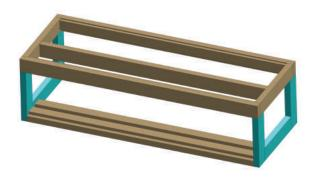
3. The leg assembly on each side of the bench is made of 2x4s screwed together with pocket hole screws.
