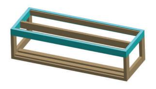
1. The top pieces of the frame should be cut to match your space. Our nook is 62 inches wide and 26-1/2 inches deep. Notice the smaller boards are cut 6-3/4 inches shorter than the nook is deep. This allows space for the front and back 2x4 as well as the decorative front frame.
