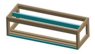
5. The top support should be recessed below the top of the bench 1/4 inch.
