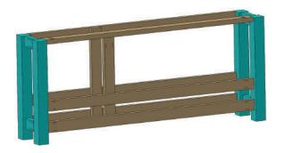
1. Each side brace (C) has 4 pocket holes drilled in it a 1/2 inch from the top and bottom edge. We used 2-1/2 inch pocket hole screws and adjusted the Kreg Jig accordingly.
