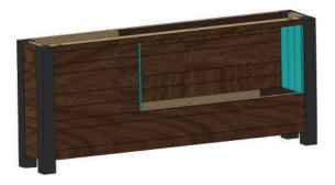
16. The inside masonite panels (M) should be attached to the three distressed wood planks (W) that line the inside of the coffee bar with 1/2 inch screws.
