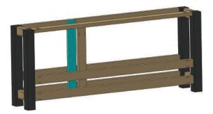
10. The back upright brace (E) is attached using 2 inch screws and is located 25-1/2 inches from the inside of the leg (A).
