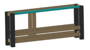
5. Each side of the top front brace (B) has 2 pocket holes drilled in it. One hole should be 1/2 an inch from the front edge and the other hole should be 2 inches from the front edge.
