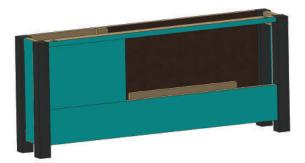
14. All the rest of the masonite panels can be attached using 1 inch finishing nails. For an extra secure hold add a bead of wood glue between the 2x4s and masonite panels.
